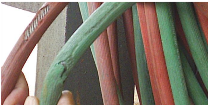
Cracked/damaged gas hose
