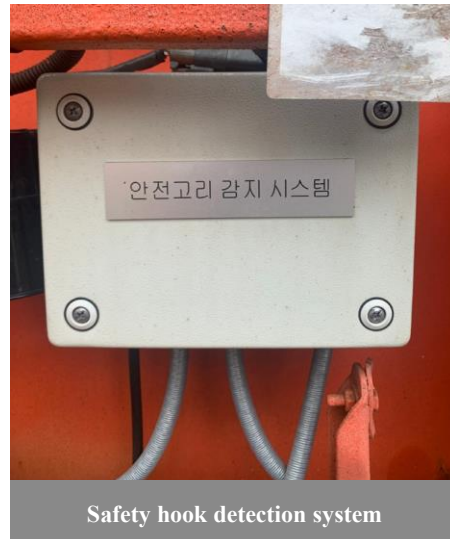
The fluorescent light is on when a hook is secured
