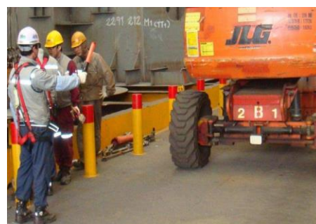
Moving the MEWP while a guide is arranged
