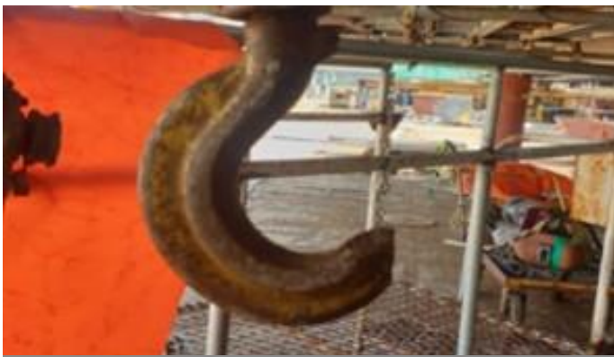
Using a lever puller with a damaged hook (e.g., broken hook end)
