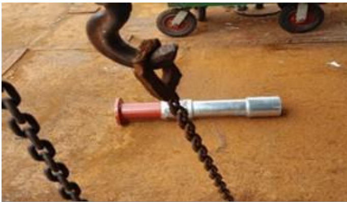
Attaching to a severely damaged lug
