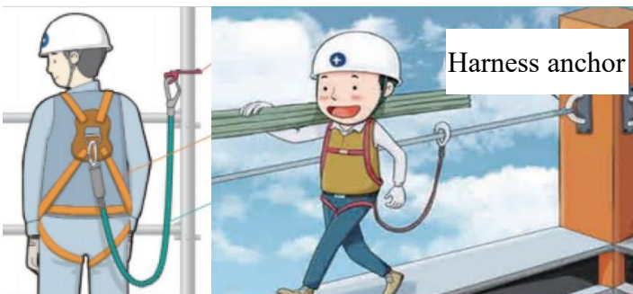
Safety harness anchoring
